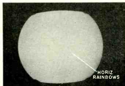
Fig. 3—Appearance of a rainbow pattern which is out of color sync.
